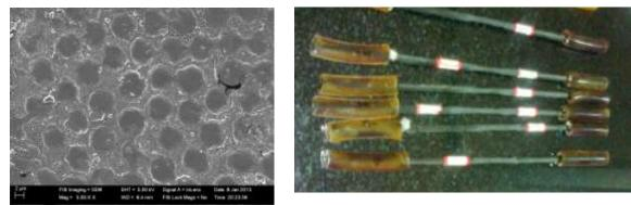
Figure 9: SEM Image of Pultruded CFRP
