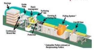
Figure 3: Schematic Diagram of the Pultrusion Process
