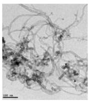
Figure 6: TEM Image of Multiwall Carbon Nano Tubes<sup>4</sup>
